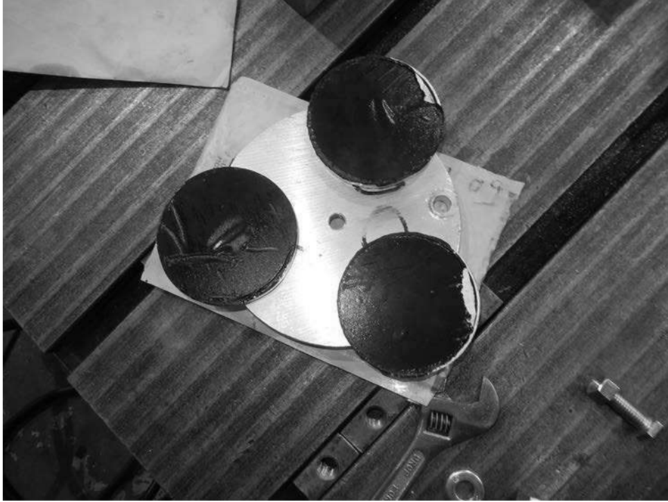
Poly pads after shear test
