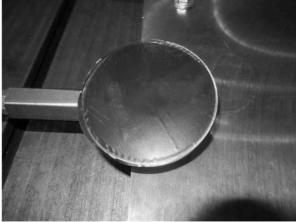
Poly pad after shear test
