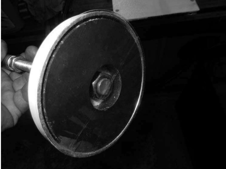
Mylar pad after tensile test
