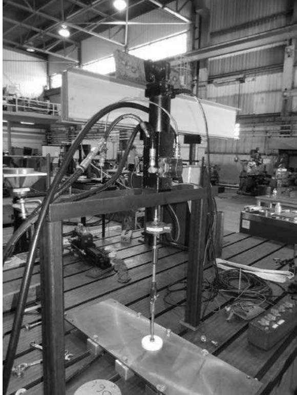
Single magnet tensile test setup on bare steel plate
